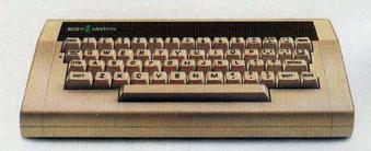
At the heart of the machine lies 64K of memory. Of this, 32K is in the form of ROM (Read Only Memory) containing the Machine Operating System and BASIC interpreter. The other 32K is RAM (Random Access Memory), over 20K of which can be available to you for writing your programs.
